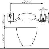
When using a back support, the distance must be 730 mm (clearance 700 mm) from the folding grab rails.
